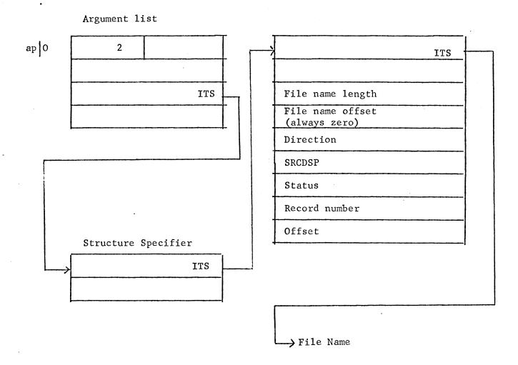
Figure 1 - Open/Close Argument List Structure (Portions of the structure not used by EFS are not shown.)
