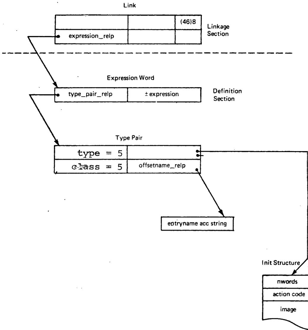
Figure 1-2. Structure of a Link
